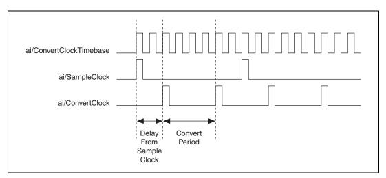
Figure 4-12. ai/SampleClock and ai/ConvertClock
